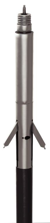
**MCR's Electro-Mechanical Anchor** is an electric line or slickline\* deployed anchoring device intended for use with MCR's systems. With outside diameters (retracted) of 1-1/2", 1-3/4" and 2-1/2", EMA's effectively anchor tools for cutting tubulars from 2-3/8" to 7-5/8". Anchor arm material and design allow for fixation within ALL tubular materials covered by MCR system specifications, e.g. Monel®, Hastelloy®, Inconel®, Chrome, and plastic coated tubulars.
